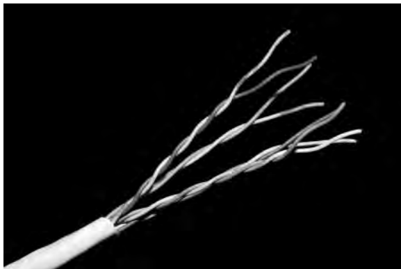
FIGURE 3.9 Category 5e twisted pair wire Source: © Jason/Alamy
