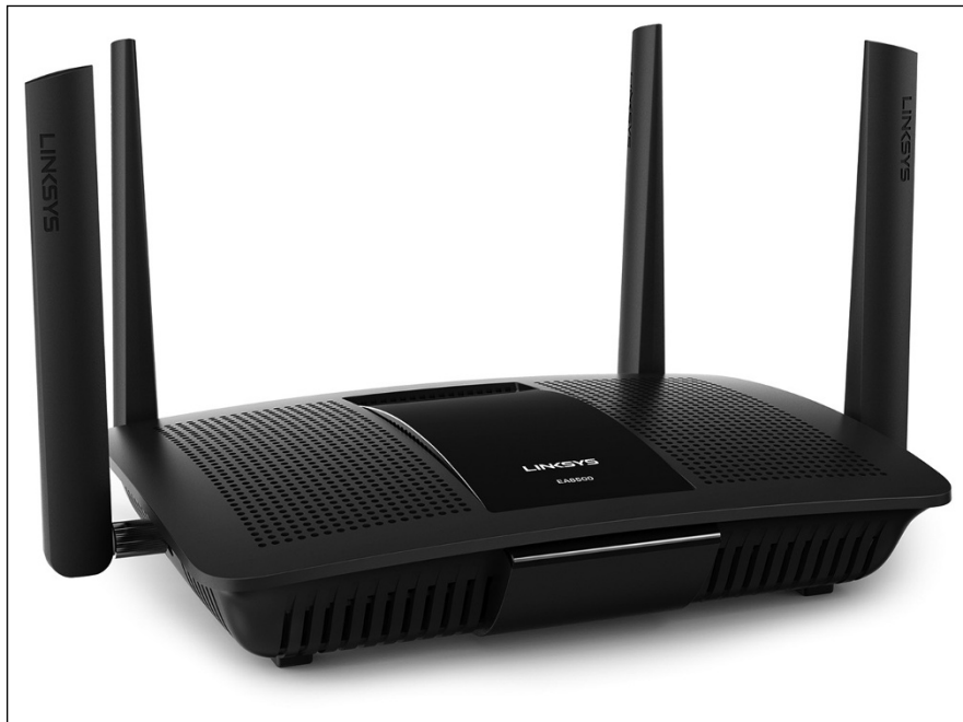
Figure 8-4: A typical wireless router.
