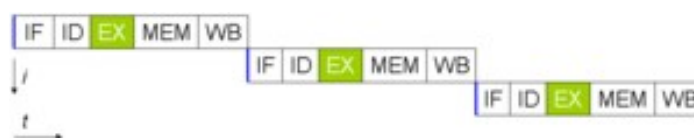
Figure 3: Non-pipelined CPU. It takes 15 cycles to complete 3 instructions
