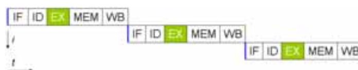
Figure 3: Non-pipelined CPU. It takes 15 cycles to complete 3 instructions
